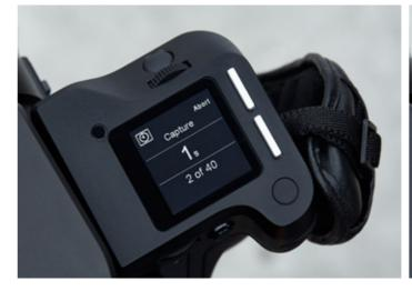
Capture Delay will pause the camera between each capture (in this case 1 second)....
