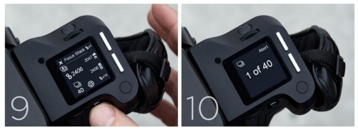
Start Focus Stack Use the rear button to start Focus Stack and capture images.
