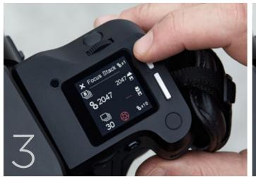
Assign the distant focus point Save the focus point with the front button.
