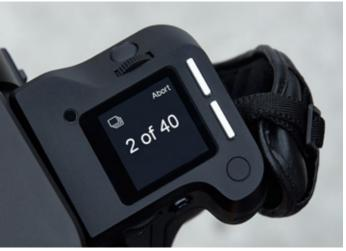
...and shoot all frames, one after another (in this case 40). Another big advantage of the Focus Stack tool is that the photographer can walk away from the camera when it's capturing images: no unwanted reflection of the photographer's hand in the subject, no unwanted vibrations either.
