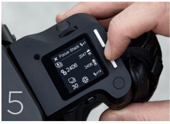
Assign the near focus point Save the focus point using the rear button.
