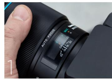
Set the lens to Auto Focus The Focus Stack tool can't operate if lens is in Manual mode.
